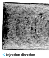
Fibers alignment rate in a composite material
